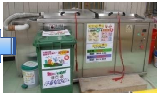
4. Wood chips were used as bulking agent to mix with food/garden waste and decomposed into soil conditioner
