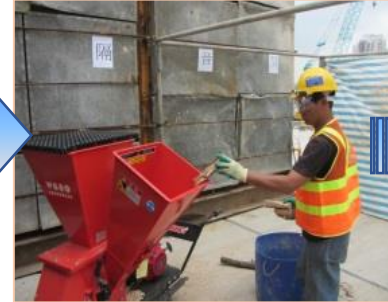
2. Felled trees were cut and shredded into wood chips
