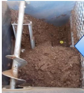
4. Wood chips were used as bulking agent to mix with food/garden waste and decomposed into soil conditioner
